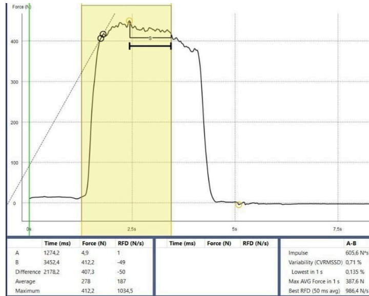
Figure 23. The figure presents the results of a finger strength test performed using the Chronojump force sensor. The analysis includes the maximum force value, rate of force development (RFD), force impulse, and the differences between measurements taken in sample A and sample B.
