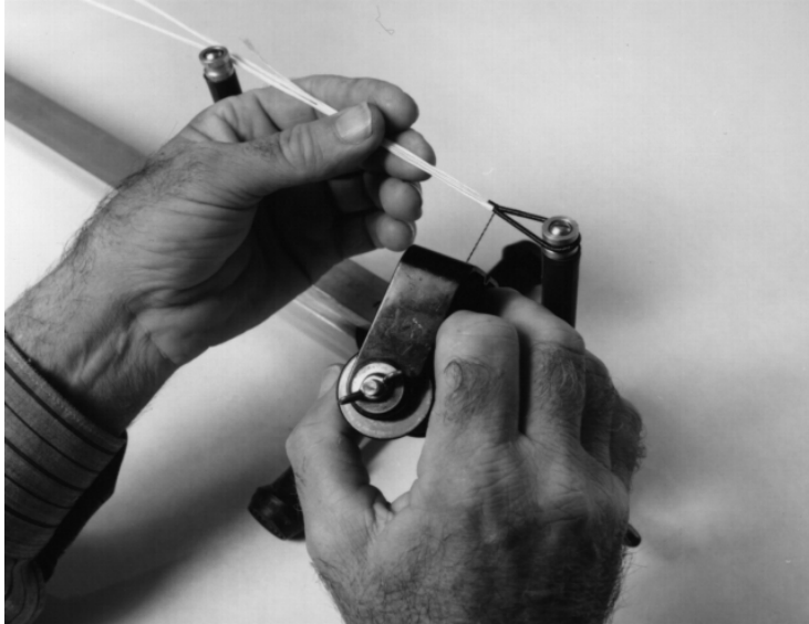
When the correct length of serving has been reached, turn the string jig posts and continue to serve
